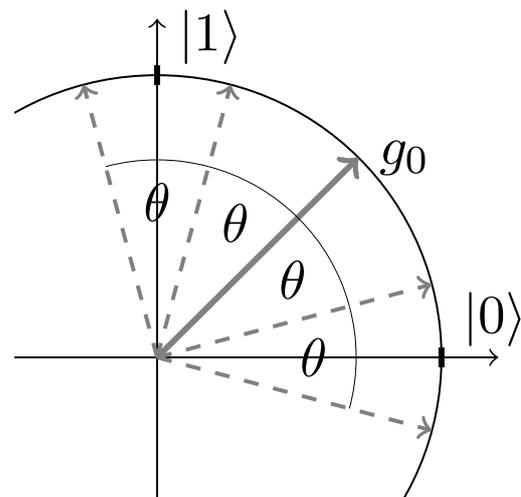
Fig. 5. The update operation based on the rotation angle  $\theta$  that divides the initial angle ( $45^\circ$ ) with a non-zero remainder is incapable of creating a state of quantum gene that has no uncertainty.
